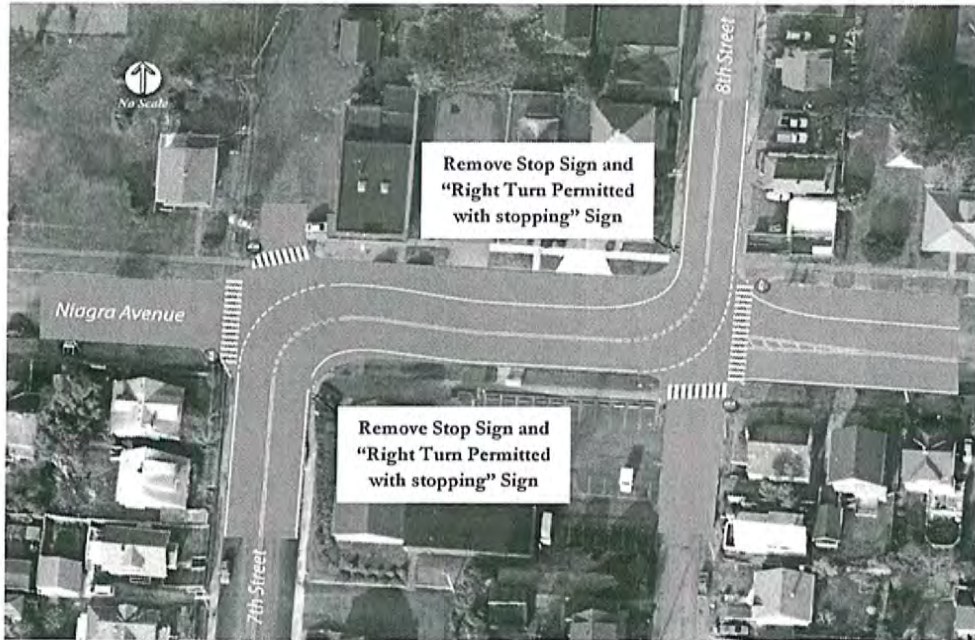
Figure 9: Potential Configuration of Niagara Avenue/7 th Street-8 th Street Intersections under Option 3
