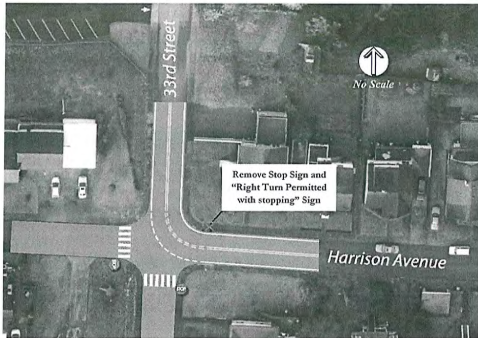
Figure 14: Potential Configuration of Harrison Avenue/33rd Street Intersection under Option 3
